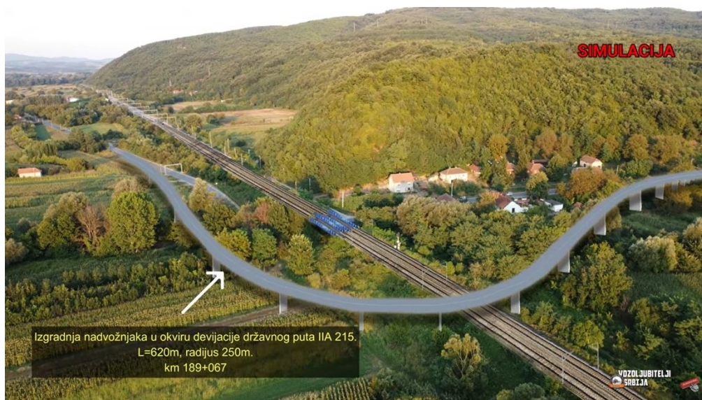
Figure 36: Route of the future railway alignment with the construction of an overpass within the realignment of the state road in the Djunis settlement
