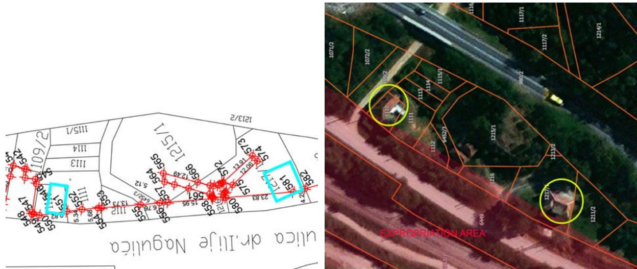
Figure 3 Example showing by how little the preliminary expropriation line cut across two houses
